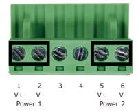
Figure 3-5: The pin of 6-contact terminal block connector
